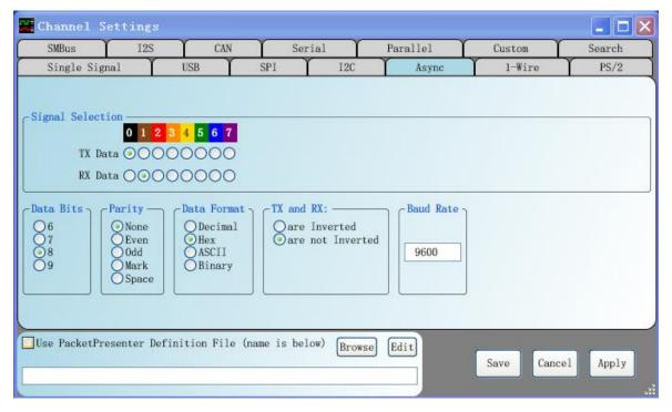
Click on the "Capture Once" sampling time interval with the mouse to adjust the signal, you can see the decoded content, you can display the hex, ASCII and other formats.
