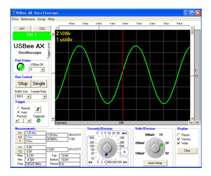
Time waveform display, you will see the trigger point. Trigger point with a red vertical dashed line and horizontal "T" shown.
